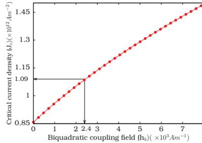
**FIGURE 2.** A plot of the biquadratic coupling field versus critical current density.
