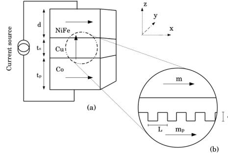
**FIGURE 1.** (a). Geometry of the Co/Cu/Ni-Fe nanopillar device. (b). In the zoomed view, we see the pinned layer (Co) have periodic interfacial terraces with a period  $L$  and a height  $\delta$ .
